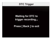
Press the [ $\sqrt{\ }$ ] to start recording or wait codes to trigger.
