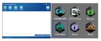
Connect the scanner to the computer via USB cable to power it on. Run the Update Tool on your computer. Select [Print]. Select [Print Data] on the OBDII scanner.
