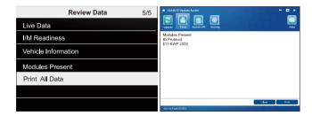
Select desired data to print. If all recorded data is to be printed, select [Print All Data]. Then press the [  $\sqrt{\ }$  ] key.
